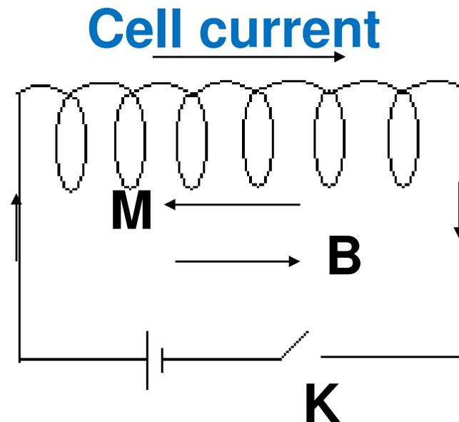
On pressing key K current through the cell increases from zero to a certain maximum value which takes some time. During this time (Make time M) current through the coil is increasing, magnetic flux linked with the coil is increasing, therefore, a current is induced in the coil. So according to Lenz's law, the induced current at the make will oppose the growth of current in the coil by flowing in the direction opposite to the direction of the cell current.
