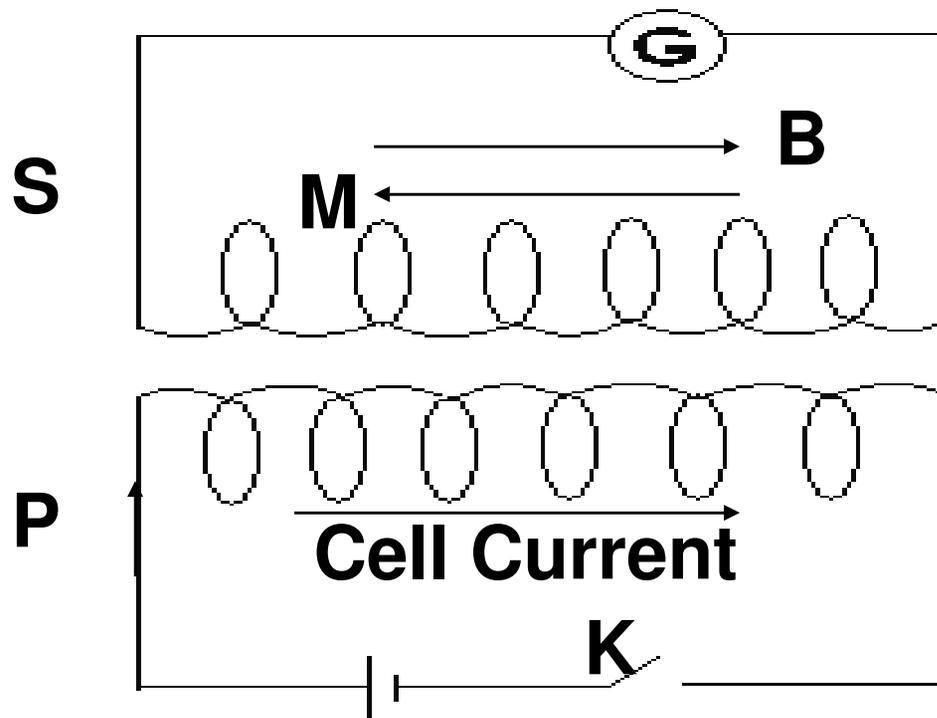
On pressing K, current in P increases from zero to maximum value. It takes some time ( Make time M) current is increasing in P, magnetic flux linked with P is also increasing. As S is closeby, magnetic flux associated with S also increases, an e.m.f. is induced in S. So, according to Lenz's law, induced current in S would oppose increase in current in P by flowing in direction opposite to the cell current in P.
