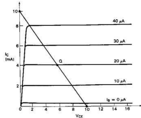
What is  $I_{C(sat)}$  and  $V_{CE(off)}$  ?
