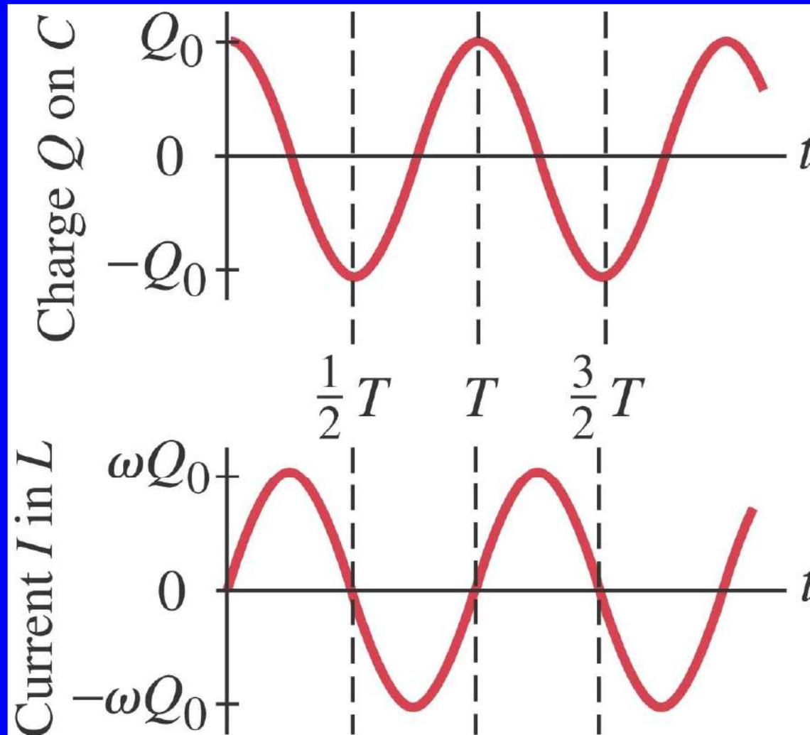
The total energy in the circuit is constant; it oscillates between the capacitor and the inductor:
