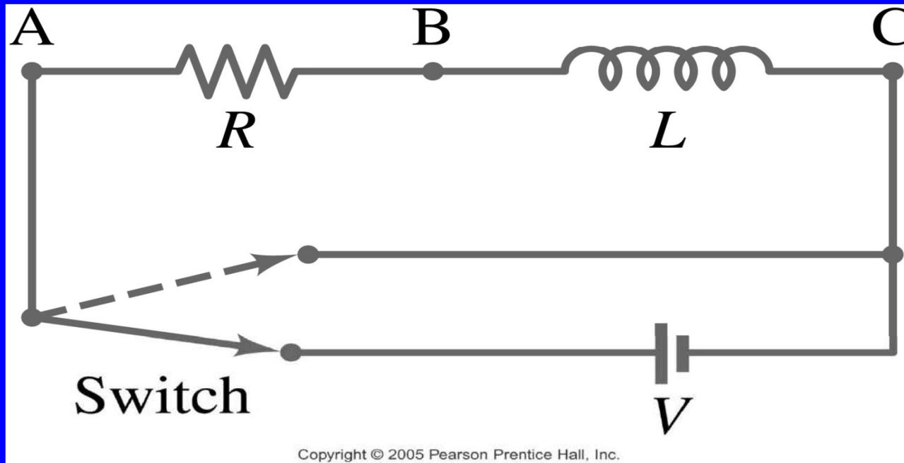
As a circuit is completed, the current begins to increase, but the inductor produces an emf that opposes the increasing current. Therefore, the current doesn't change from 0 to its maximum instantaneously.
