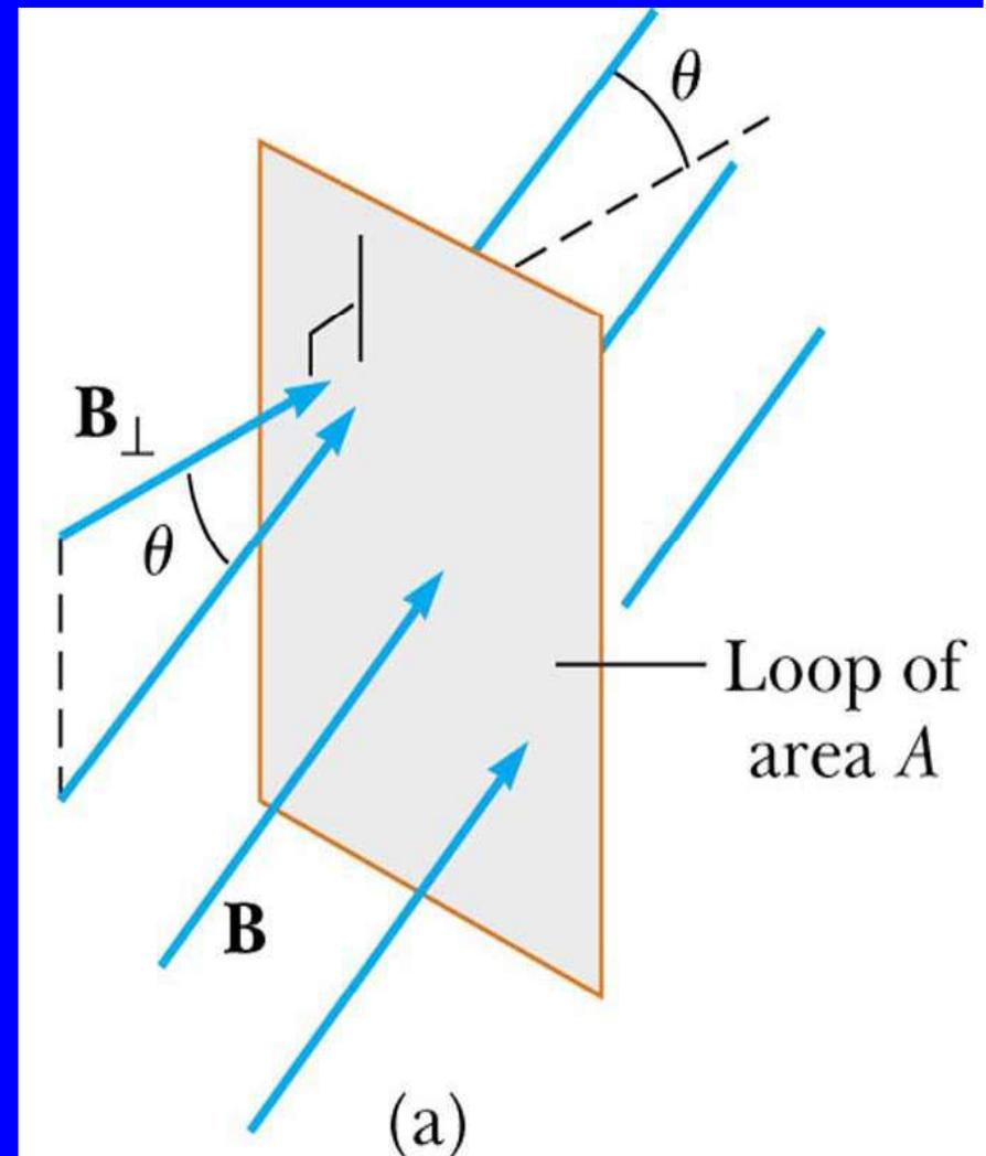
The induced emf in a wire loop is proportional to the rate of change of magnetic flux through the loop.
