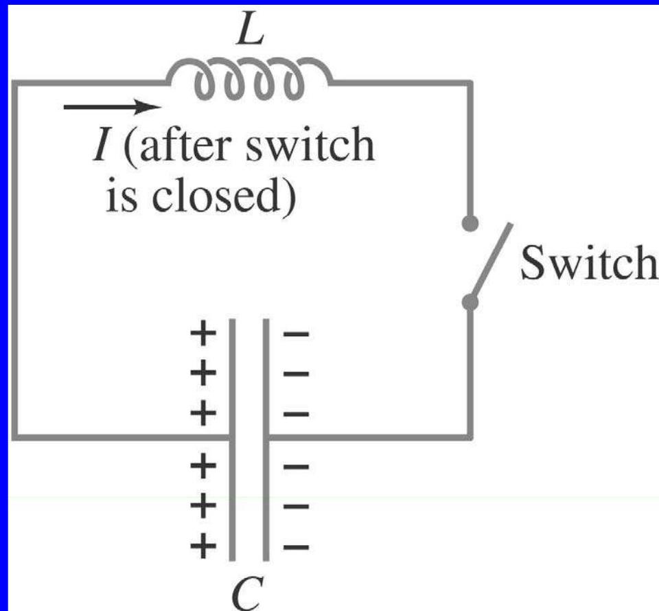
Summing the potential drops around the circuit gives a differential equation for  $Q$ :
