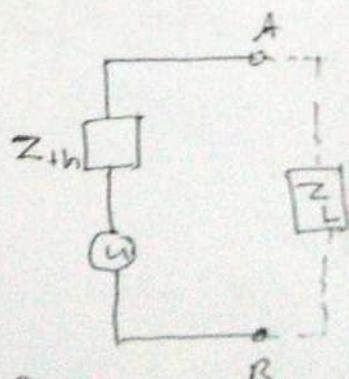
$N$  is a network containing a number of sources and linear impedances with output terminals  $A$  and  $B$ . Let  $E_{th}$  be the open-circuit voltage
